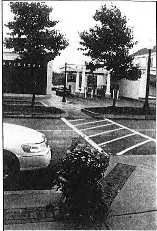
Elements of a pedestrian oriented streetscape include curb bump-outs, crosswalks, planted medians and sidewalks. As an alternative to tradition striped crosswalks, materials such as concrete, brick or pavers, may be used to further emphasize pedestrian areas such as crosswalks within a roadway.
